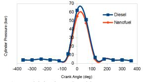
Figure 1: Variation of cylinder peak pressure for nanofuel.
