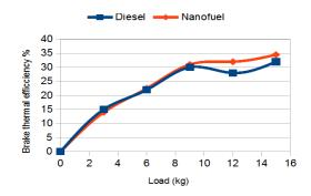
Figure 4: Brake thermal efficiency vs. load
